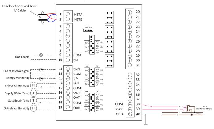
Note; All inputs are universal inputs. Consult the application guide for proper dip switch configuration
