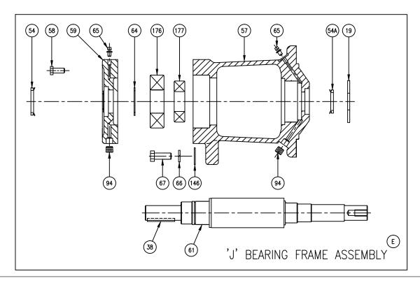
NOTE: Note difference in visual appearance of bearing frames on pages 3 and 4. New frames are a direct replacement for older ones. The part numbers for individual bearings are different from old frames to new frames. If you need help determining which frame you have, please contact tech services at Taco (401-942-8000).
