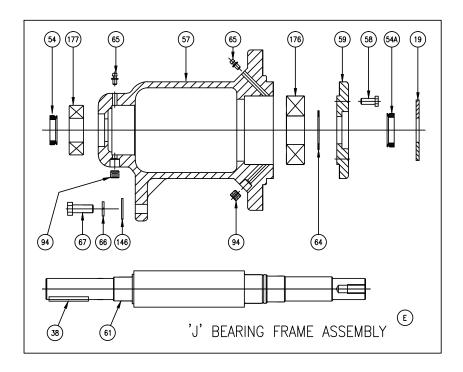
NOTE: Note difference in visual appearance of bearing frames on pages 3 and 4. New frames are a direct replacement for older ones. The part numbers for individual bearings are different from old frames to new frames. If you need help determining which frame you have, please contact tech services at Taco (401-942-8000).
