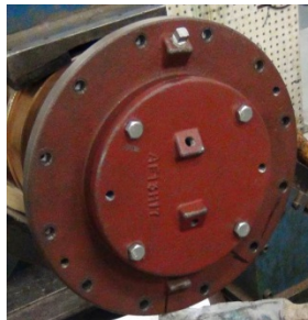
Cover Attached to Bearing Housing with Correct Grease Hole Orientation
