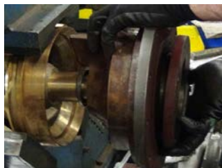
Bearing Housing and Cap Placed on Impeller Shaft
