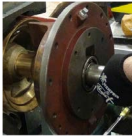
Slide Bearing onto Impeller Shaft
