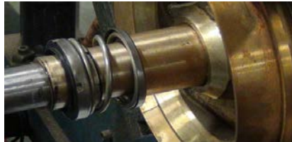
Mechanical Seal Assembly on Sleeve
