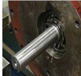
Lock Washer against Bearing on Impeller Shaft
