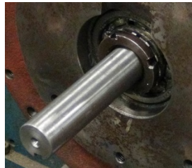
Bearing Retainer Nut against Lock Washer
