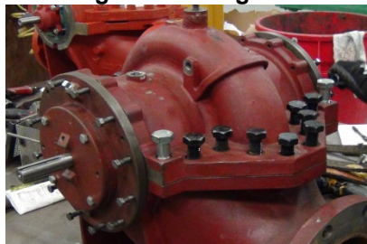
Casing Cover Reattached to Casing bas with all Bolts
