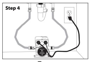
Plug in the circulator and it will start automatically, run until hot water is detected by the temperature sensor, and then stop. Set up is complete you are ready to enjoy hot water comfort. **8** mins Time delay of motion sensor
