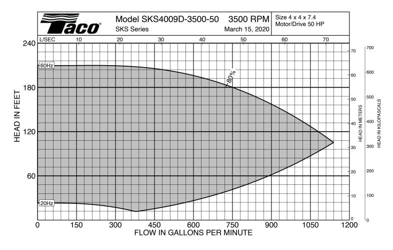
Curves based on Clear Water @ 60F with a Specific Gravity of 1.0
