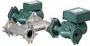
The modified RMB, called the LOFlo Mixing Block (LMB), circulates water to the terminal units. The LMB consists of a zone circulator for water flow through the secondary circuit to the terminal units, and a variable injection pump that takes a signal from the BAS to inject cold water to always maintain the above dew point system temperature.
