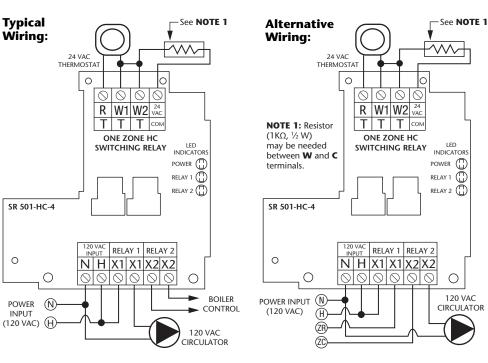
**NOTE 2:** When using Alternative Wiring diagram, the boiler operating control's ZC terminal will see the load of the circulator(s).
