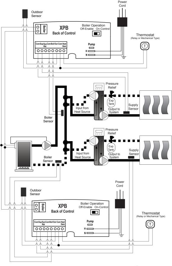
X - Pump Block (XPB), Multiple Temperature System
