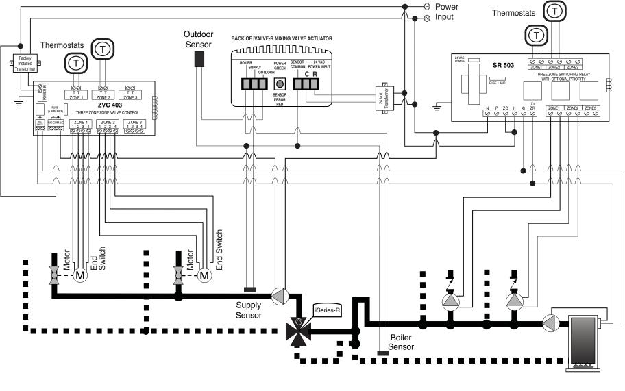
iValve 4-way Mixing, Multiple Temperature System
