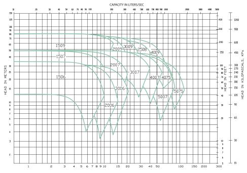
FLOW IN GALLONS PER MINUTE • 2900 RPM • KV QUICK SELECTION CURVE
