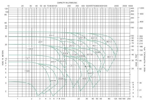
FLOW IN GALLONS PER MINUTE • 1450 RPM • KV QUICK SELECTION CURVE
