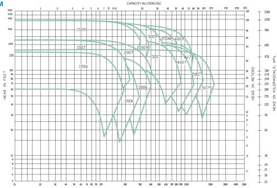
FLOW IN GALLONS PER MINUTE • 3500 RPM • KV QUICK SELECTION CURVE
