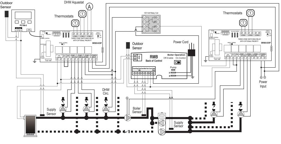
RMB - Radiant Mixing Block, Multiple Temperature System with DHW Priority and Boiler Reset
