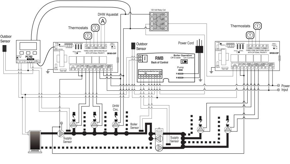
RMB - Radiant Mixing Block, Multiple Temperature System with DHW Priority and Boiler Reset
