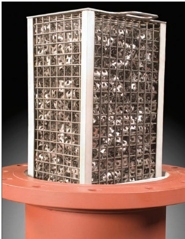
*The PALL Ring chamber optimizes a collision of flowing system water with the PALL Rings. As a result, all of the gas-containing water particles are brought into contact with the entire PALL Ring surface area. Even the smallest microbubble present in the water adheres to the surface of a PALL Ring, allowing coalescence to occur and air to be removed.*
